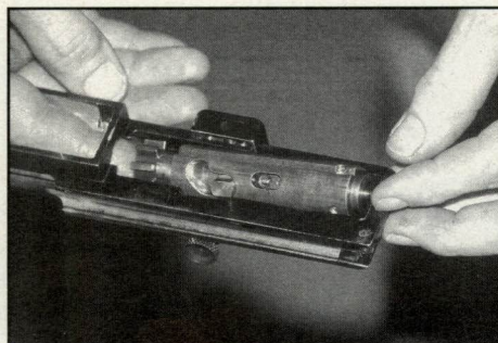
Reed Knight removes bolt carrier assembly from Stoner prototype M5.
