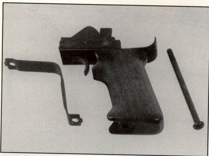
Stoner prototype M8 pistol grip/trigger group showing trigger guard and assembly bolt.
