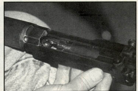
Stoner prototype M5 locking lugs compared to barrel extension.
