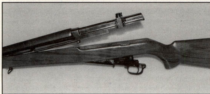
2. Lifting upper receiver, lowering trigger assembly.
