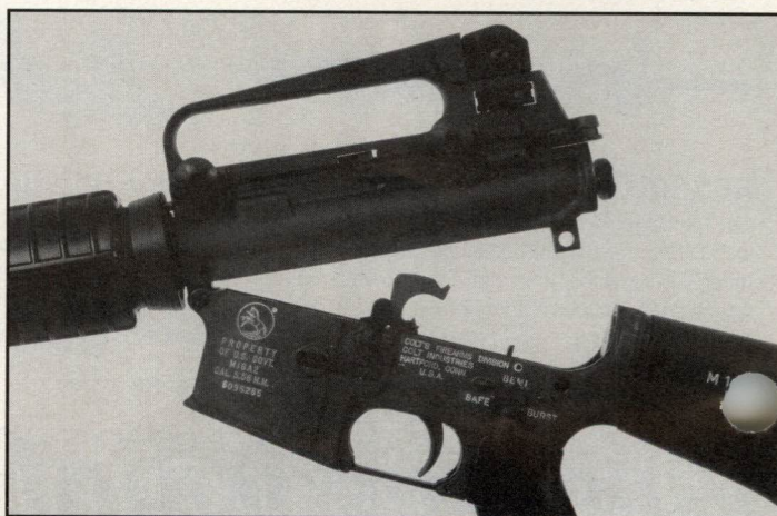
M16A2 (enhanced). The M16 at the other end of the evolution. Upper and lower opened for inspection.
