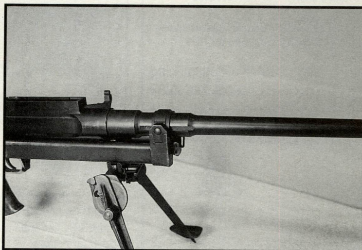
Below: Picture 8: Barrel assembly slides under recoil in the support ring.
