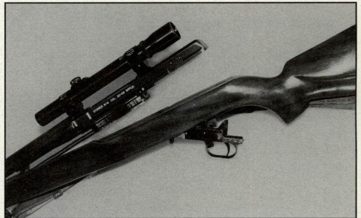
Upper receiver raised from stock, hinged trigger group in down position. Note: the new design hinges the trigger group at the rear of the magazine well.
