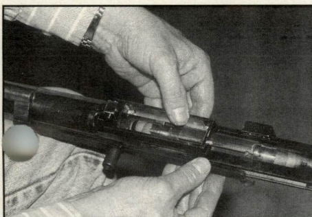
Removal of operating rod showing light recoil damage to aluminum receiver guiding rails.
